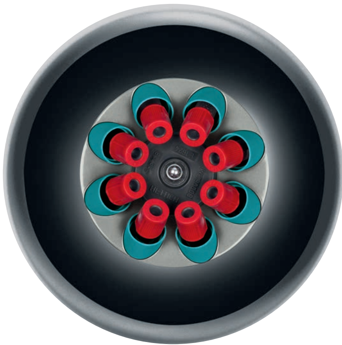
View into the centrifuging chamber showing the rotor with blood collection tubes
